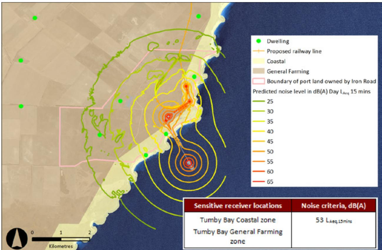
Figure 12-9 Predicted Operational Noise Contours for Proposed Port Development, Day  $L_{Aeq,15mins}$
