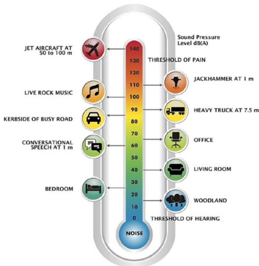
Figure 12-1 Some Examples of Typical Sound Levels in dB(A)
